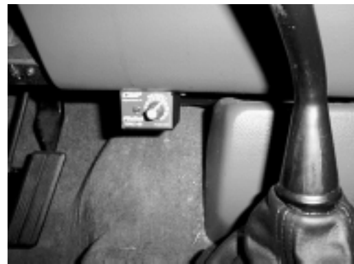
Figure: 9B-b Timing Retard Control Knob.
