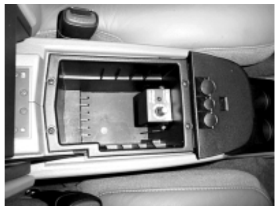
Figure: 9A-e Install Center Console and Tray.
