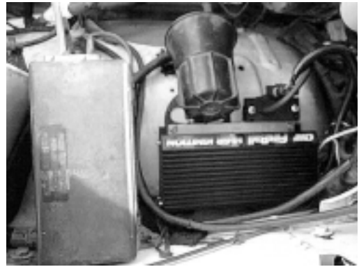
Figure: 9B-a Mounting Ignition Box.
