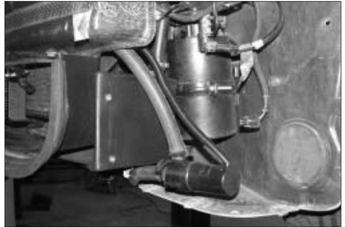
*Fig. 9-d.1* / (1992-1995 Model Year Reservoir Mounting)
