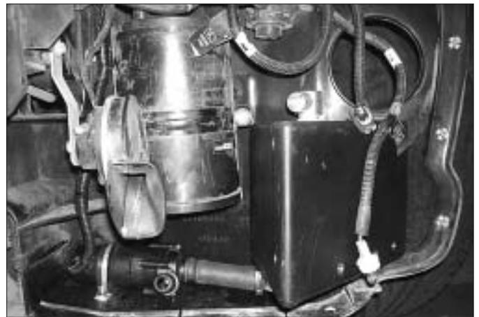
*Fig. 9-d.2* / (1996 Model Year Reservoir Mounting)
